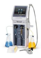
The Dual Syringe Dispenser has two syringe drives for applications such as Animal Dosing that require the use of more than one liquid at the same time. The two liquids can be dosed from the same instrument saving setup and dosing time.
