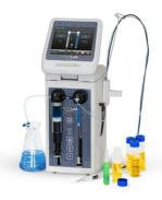
The Microlab 600's Dual Syringe Diluter configuration uses two syringes to create up to a 1:50,000 dilutions in a single step, drastically reducing preparation time and wasted reagent. The diluent washes the tubing between each sample, minimizing carryover.
