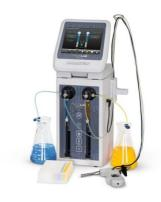
The Dual Syringe Dispenser has two syringe drives for applications such as Animal Dosing that require the use of more than one liquid at the same time. The two liquids can be dosed from the same instrument saving setup and dosing time.
