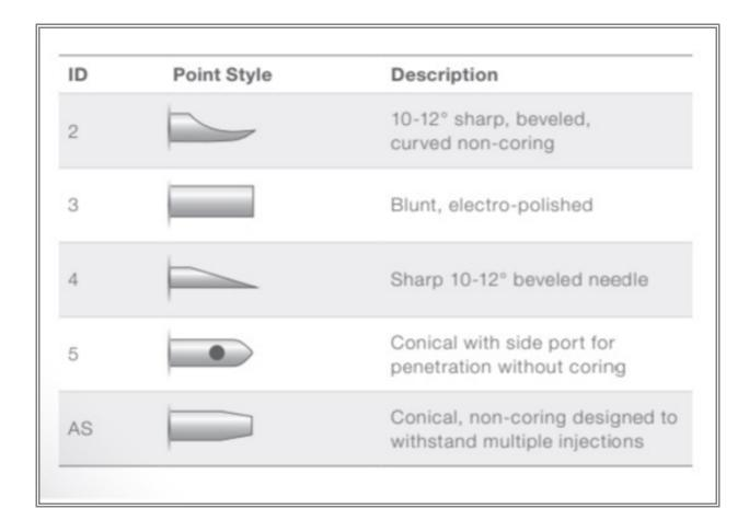
Note: For Point Style 4, please advise the degree required. Standard 12° beveled needle point is recommended for life science applications. Available gauges: 34-10. Special point styles such as 30°, 45°, or other angles between 12-60° are available upon request.
